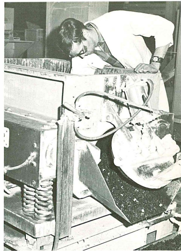
Chuck Williford, a Lorco Lab Technician, removes media from a 10 cubic foot Dual Shaft vibratory machine.
